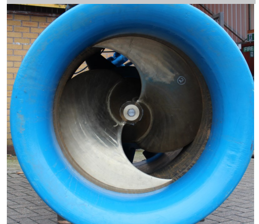
Bedford Pumps Fish Friendly Impeller
