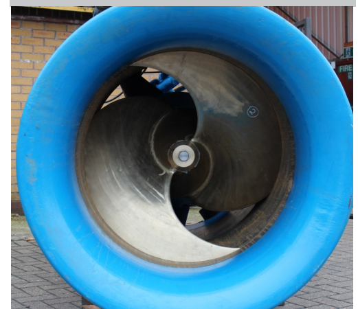
Bedford Pumps Fish Friendly Impeller
