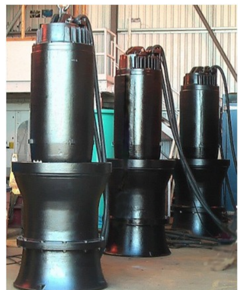
Fig 2. Bedford Pumps submersible axial pumpsets similar to those used at Pinkston
